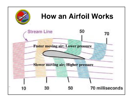
1c. Explain how an airfoil generates lift, how the primary control surfaces (ailerons, elevators, and rudder) affect the airplane's attitude, and how a propeller produces thrust.
